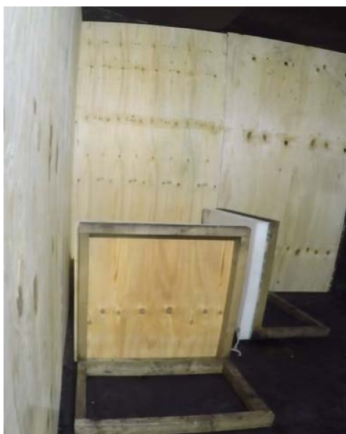
Photographs of ignition and fuel package before test 1
